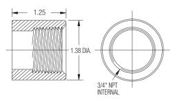
**65187 Half Coupling** - Mount to Reservoir. For use with all bulb wells shown above.
